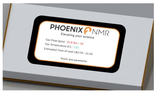
The touchscreen interface allows easy control and monitoring of the VT gas output temperature, flow rate and liquid nitrogen level.
